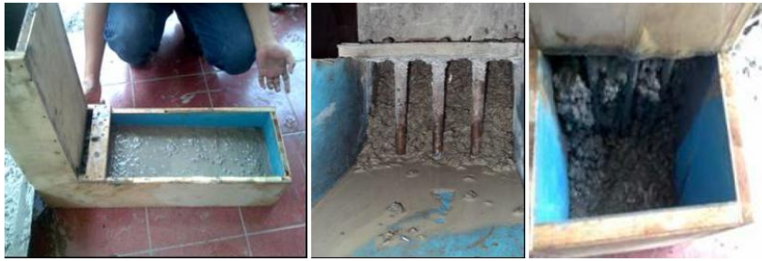
(a) SCC with 1% fine tire fibre (b) blocking SCC 1% cans fibre (c) blocking on U-box test
