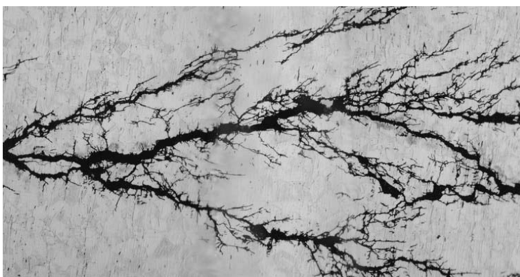
Fig 10- The photo above shows the cross section of the stress fracture (stress corrosion is usually branched) [4]
