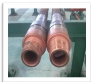
Fig 4- Drill rods attached to drill
