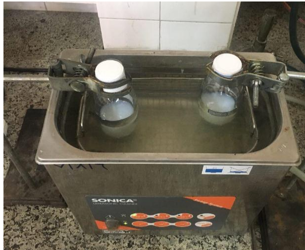
Figure 5- TiO 2 nanofluids under sonication by bath sonicator
