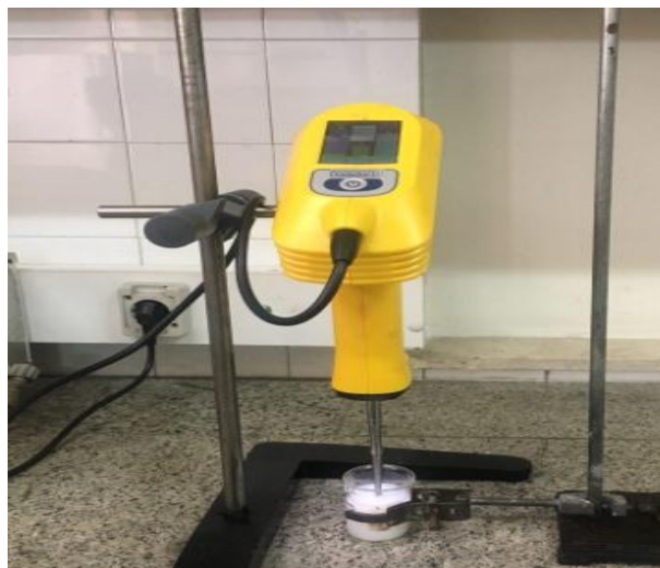
Figure 4 - TiO 2 nanofluids under sonication by probe sonicator
