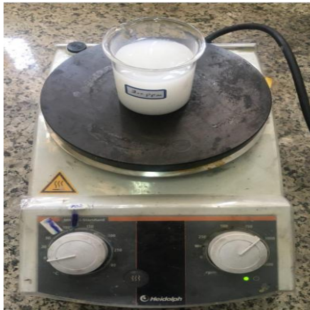
Figure 6 - TiO 2 nanofluid after 4 weeks
